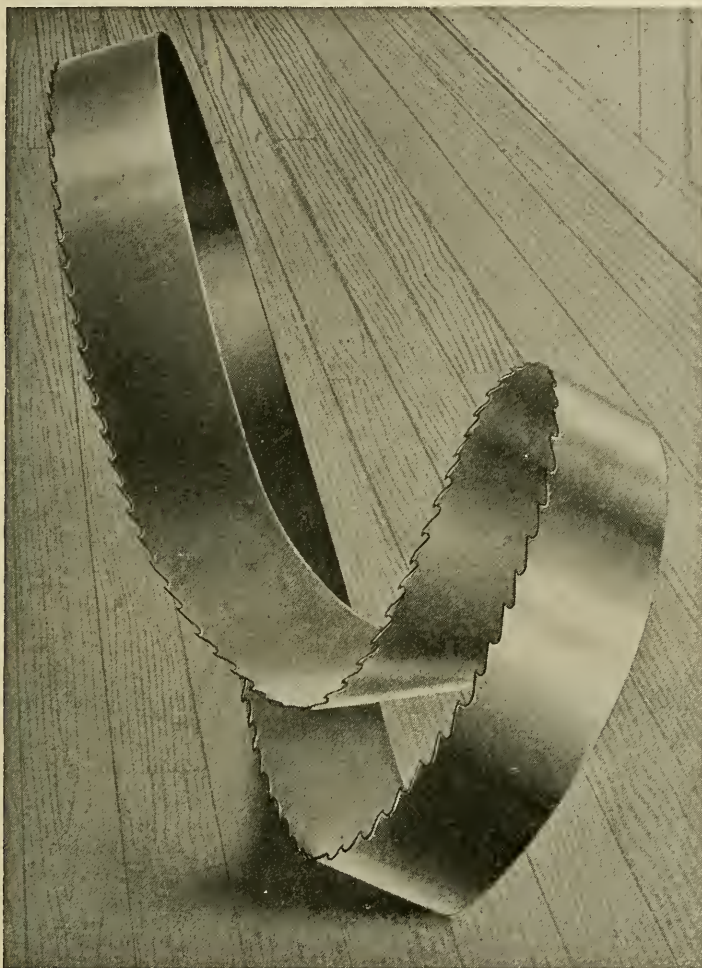
Fig. 99. This shows a band saw with a cross face twist.
