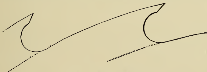
Fig. 31. Teeth for soft wood
