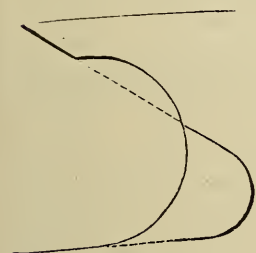
Fig. 28. Showing old and gullet style tooth
