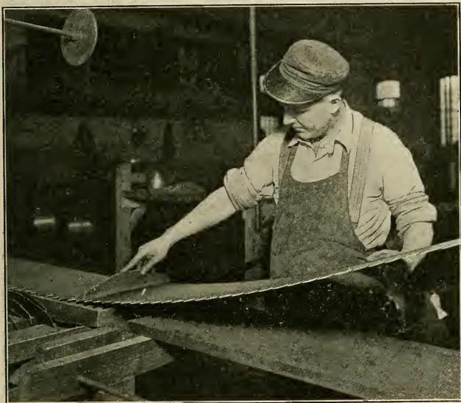
Fig. 91. "Drop" in blade fits tension gauge
