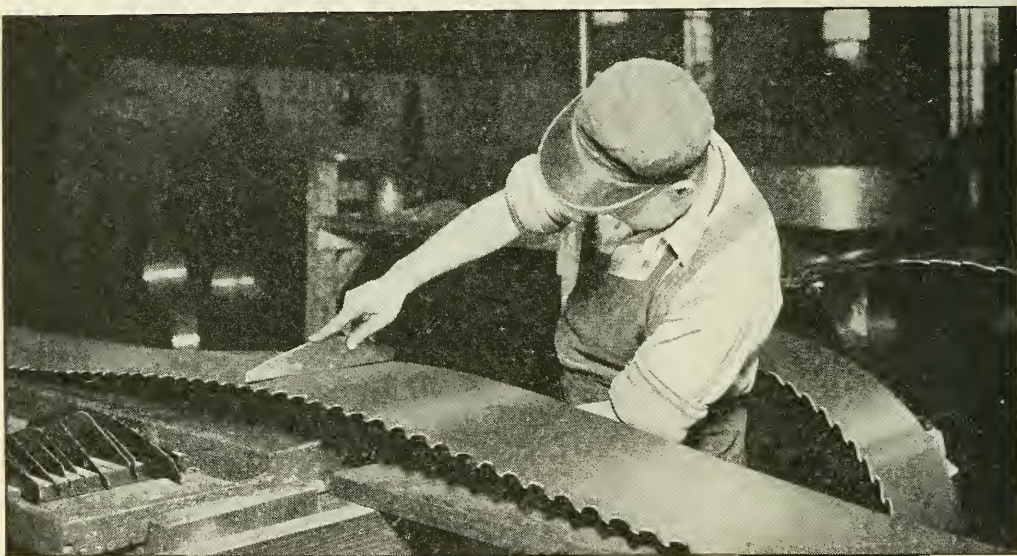
Fig. 95. Testing tension on the up-bend
